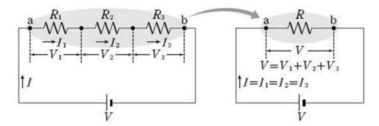
Connecting three resistors R1, R2, and R3 in sequence is called a series connection of resistors.
