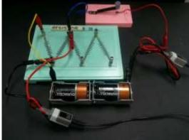
4. Finally, connect the voltage sensor to points a and c to measure the voltage across R1 and R2 together, and measure the current in the circuit with the current sensor..
